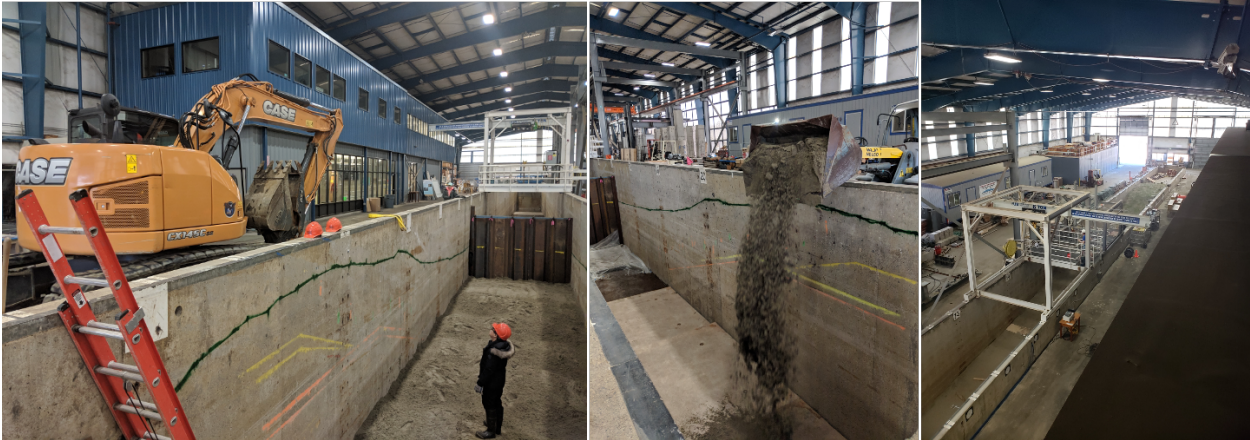
Fig. S6. The dune sand was placed in the LWF in Corvallis, Oregon.
