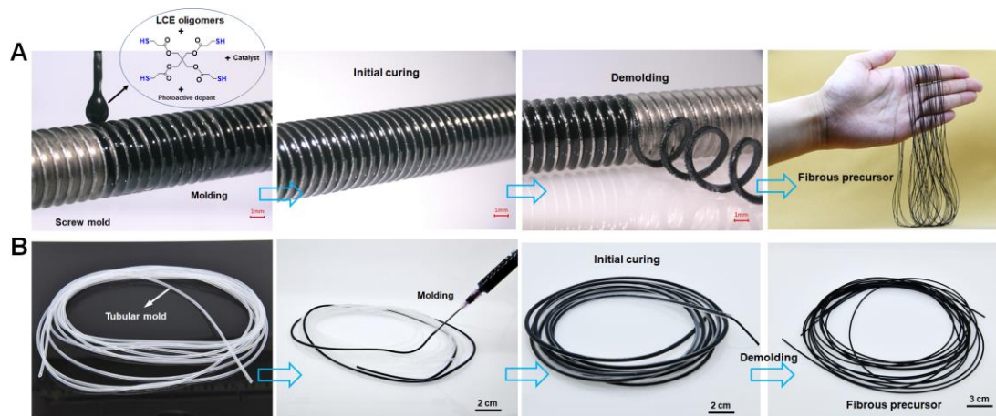
Fig. S2. Preparation of the fibrous precursors for modular fabrication of HAFMS-TSAs. (A) Experimental photographs showing the processing procedures using the screw mold to produce the fibrous precursors. (B) Experimental photographs displaying the fabrication procedures using the tubular mold to gain the fibrous precursors.
