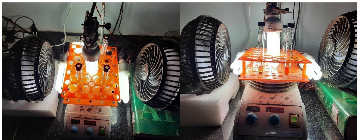
Figure S1: Photograph of the light set used for irradiation of the reaction solutions
