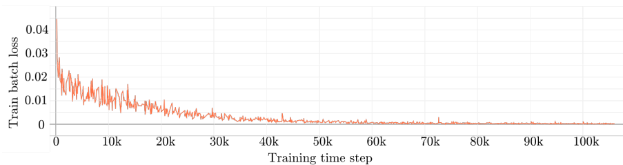
Fig. 1 Training loss curve. The loss used to train the network is a linear combination between the Dice similarity coefficient and binary cross entropy L = \frac{1}{N} \sum_1^N (1 - DSC + BCE) .
