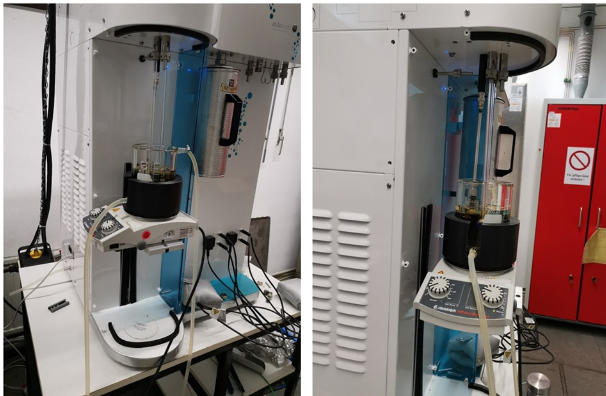
Supplementary Figure 1: Quantachrome Autosorb iQ MP instrument and the setup used for gas uptake measurements of PLs.
