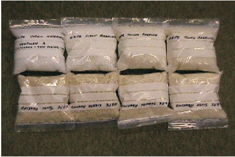
Fig. 2. The colour change in HDPE can be clearly seen after 10 process cycles. Virgin material (top left), material injection moulded and re-granulated 10 times (bottom left).
