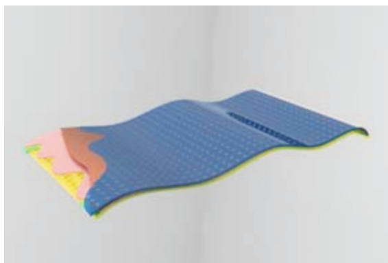
Figure 3 Image of non-ITO based flexible organic PV cell (Image from Hiflex project).
