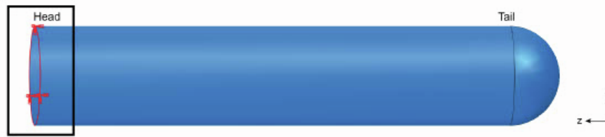
Fig. S7: Boundary conditions for the FE model, related to Figure 3. The model was constrained by imposing an encastre at the head side (black square) simulating its attachment to the brain tissue in the Drosophila embryo.
