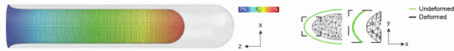
Fig. S8: Loading the FE model with a uniform pressure, related to Figure 3. Simulating loading with a perpendicular uniform pressure on the VNC resulted in its anisotropic reduction in length from tail to head (left panel). However, reduction in both the height and width of the cross-section was also observed (right panel), diverging from experimental evidence. Colours represent the magnitude of displacement along the length of the tissue (z-axis) with values ranging from 0% to 25% of strain.
