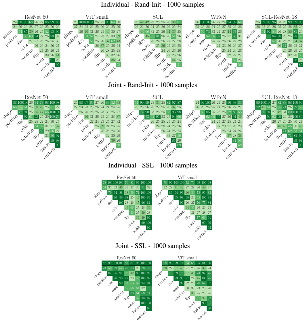
Figure 8: Task difficulty : Average accuracy on the elementary rules and their pair-wise compositions. Individual vs. Joint : Models are trained on each rule separately or trained jointly on all rules. Rand-Init vs. SSL : models are randomly initialized or pretrained with self-supervision.
