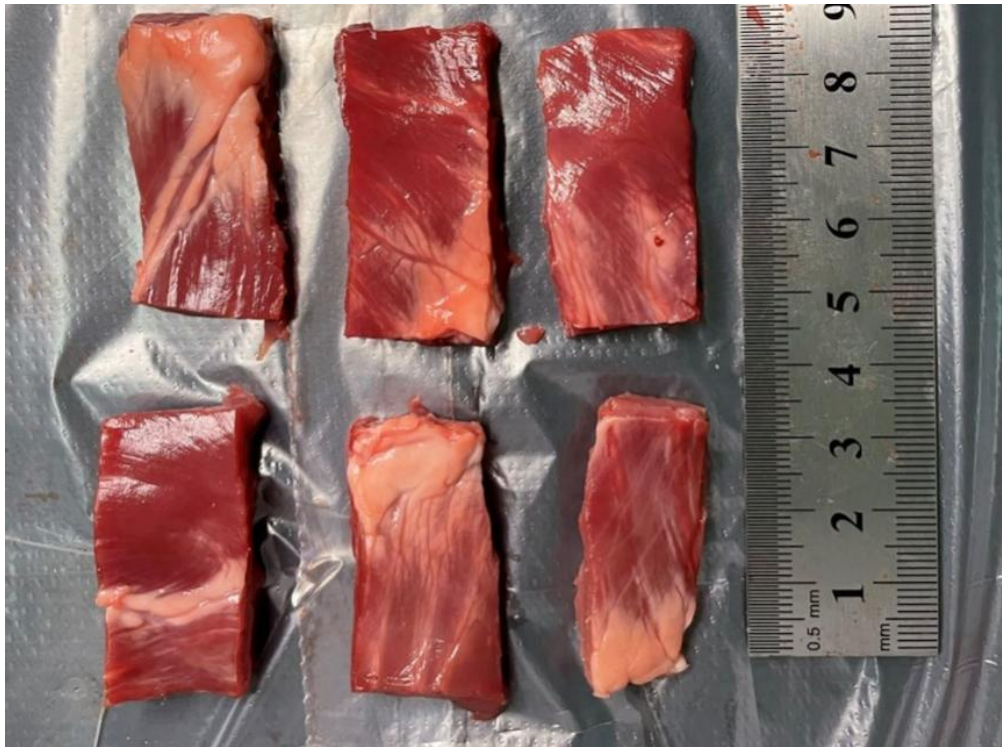
Fig. S5. The gross images of porcine heart tissue were cut into 15 mm × 30 mm × 6 mm pieces for the lap-shear tests.
