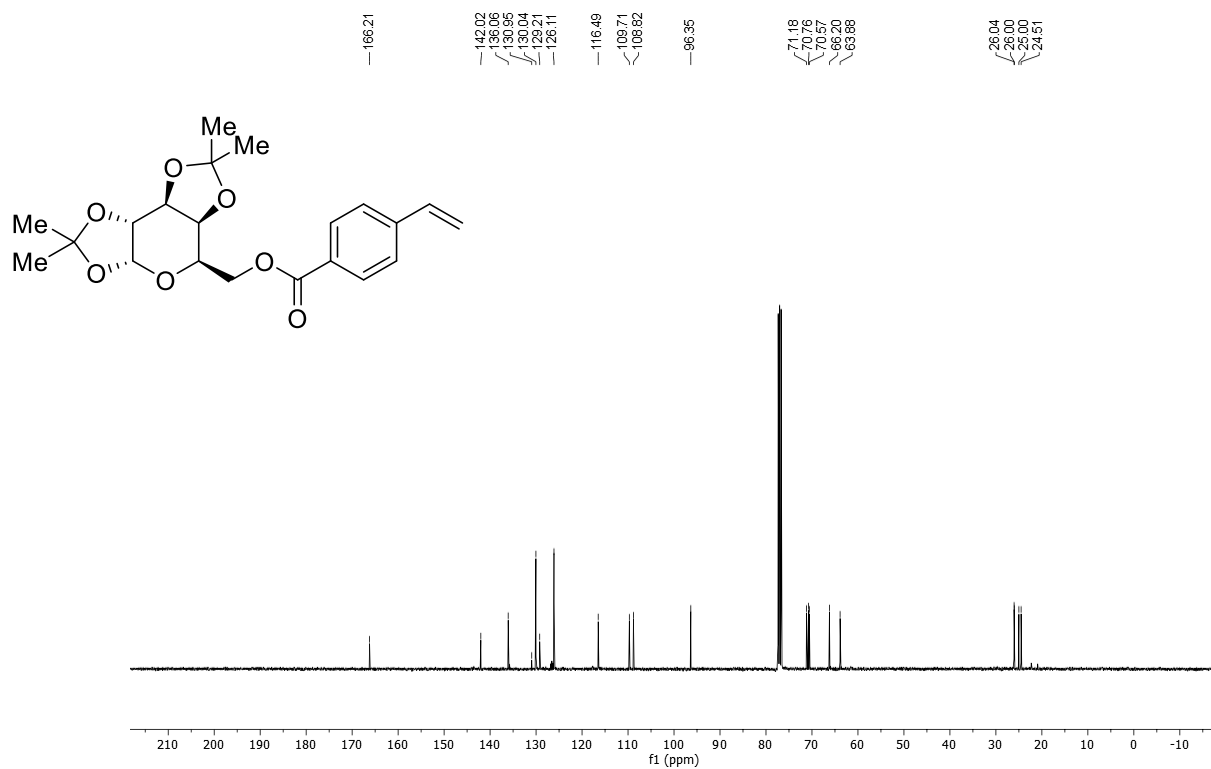
^{13}\text{C} NMR (101 MHz, \text{CDCl}_3 ) of compound 1p .
