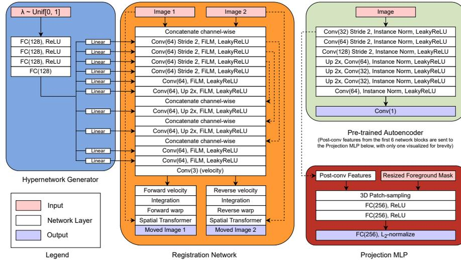
**Fig. 1. Low-level architectures** used in this paper. Connections between the registration network, autoencoder, and projection MLPs correspond to Figure 1 in the main text. Every convolution uses a 3x3x3 kernel size. LeakyReLU slopes set to 0.2.
