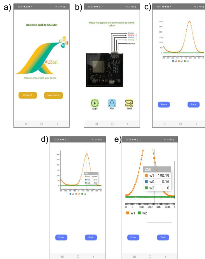
Figure S9. Screenshots of KAUSTat app control with (a) connection screen, (b) control screen, and (c) data visualization screen (d) data visualization screen with measured w_0, w_1, w_2 values (e) zoomed data screen. The peak current or other features of the curve are not calculated in the app, the user can only zoom the graph or select the values of the curve. The image created can be saved by copying the image and the data is sent by email in .txt file format. The mobile application is used only for early visualization, the data can be further post-processed and visualized in third-party software.
