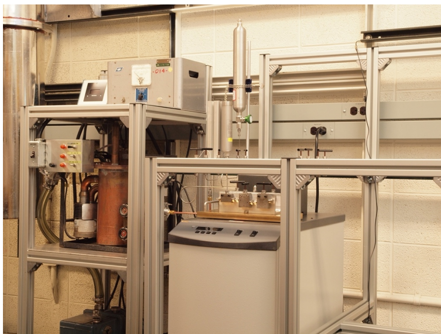
Fig. S4 Photograph of the thermostatic bath and pressure/filling manifold; the vacuum system is to the left..
