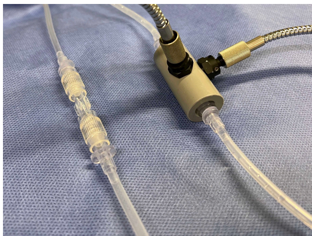
Supplementary Figure S18: Luer-to-Luer connector to measure creatinine in waste dialysate, once with clamp-on probe and once without
