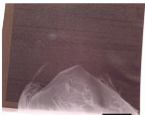
Figure S6. Calcium ion solution and electrodeposition gelation result after 1-min washing process. Scale bar: 1 cm.
