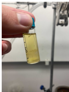
Figure S2. Reactions catalyzed by (\eta^3\text{-}1\text{-}t\text{Bu-indenyl})\text{Pd}(\text{NHC})\text{Cl} remain pale yellow, giving no indication of nanoparticle formation.
