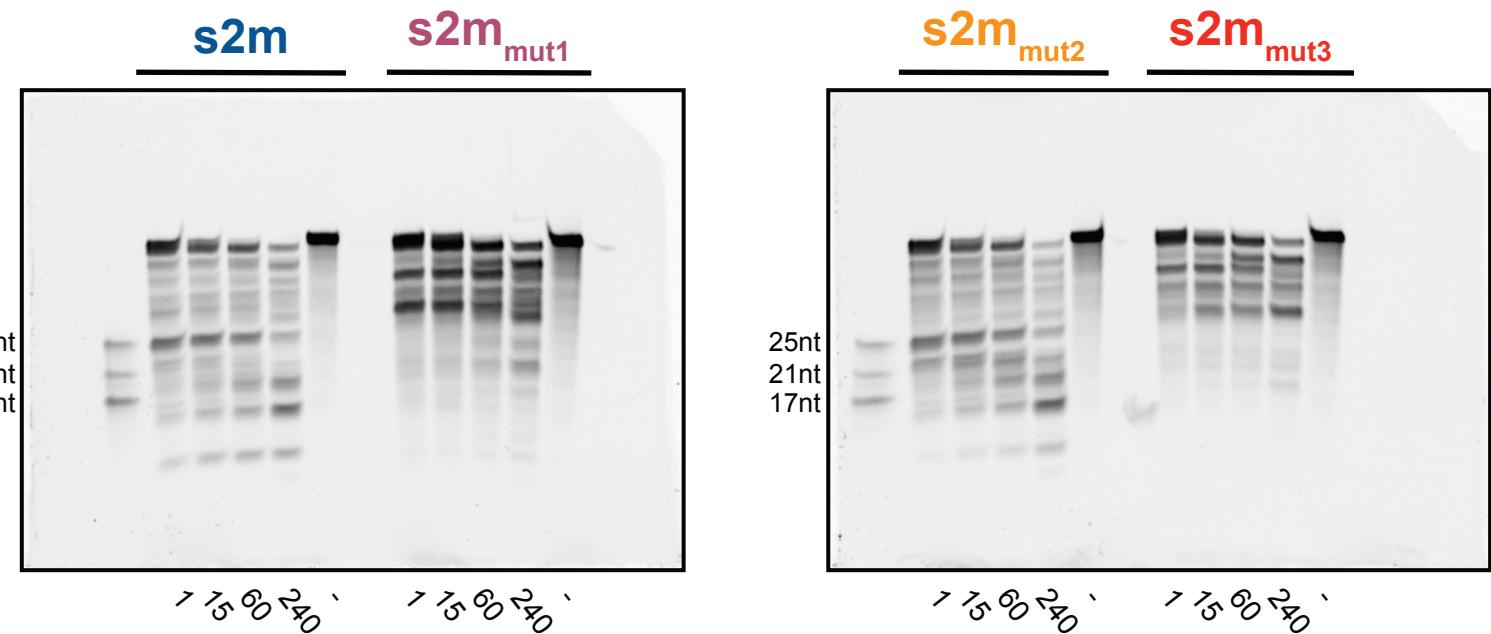
Uncropped gel for Fig 2D. Gel was captured with BioRad GelDock+ using the SYBR Green protocol.
