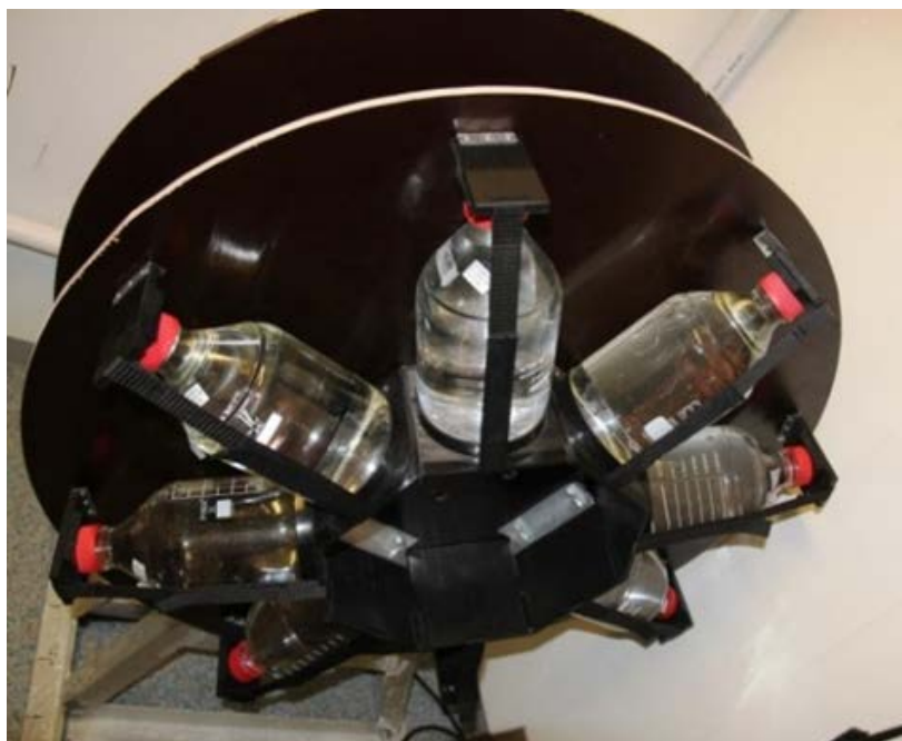
Figure S2. Incubation system comprising 2.3 L Pyrex bottles on slowly rotating (0.75 rpm) carousels in the dark at 13 °C.
