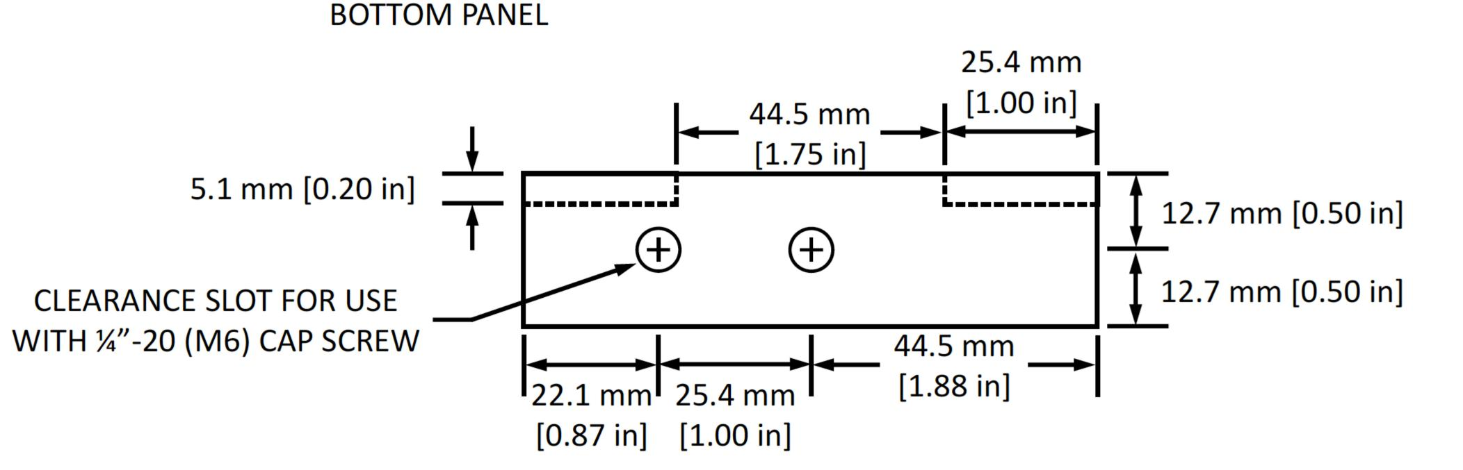
**Supplementary Figure 1.** Dimensions of the custom-made capillary holder. The figure is drawn to scale.
