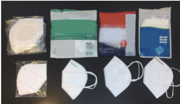
Figure S11. Material information and calibrator. (A) N95 and KN95 respirators. (B) Digimatic digital calipers were used to measure the thickness of the outer, filter, cotton, and inner layers.
