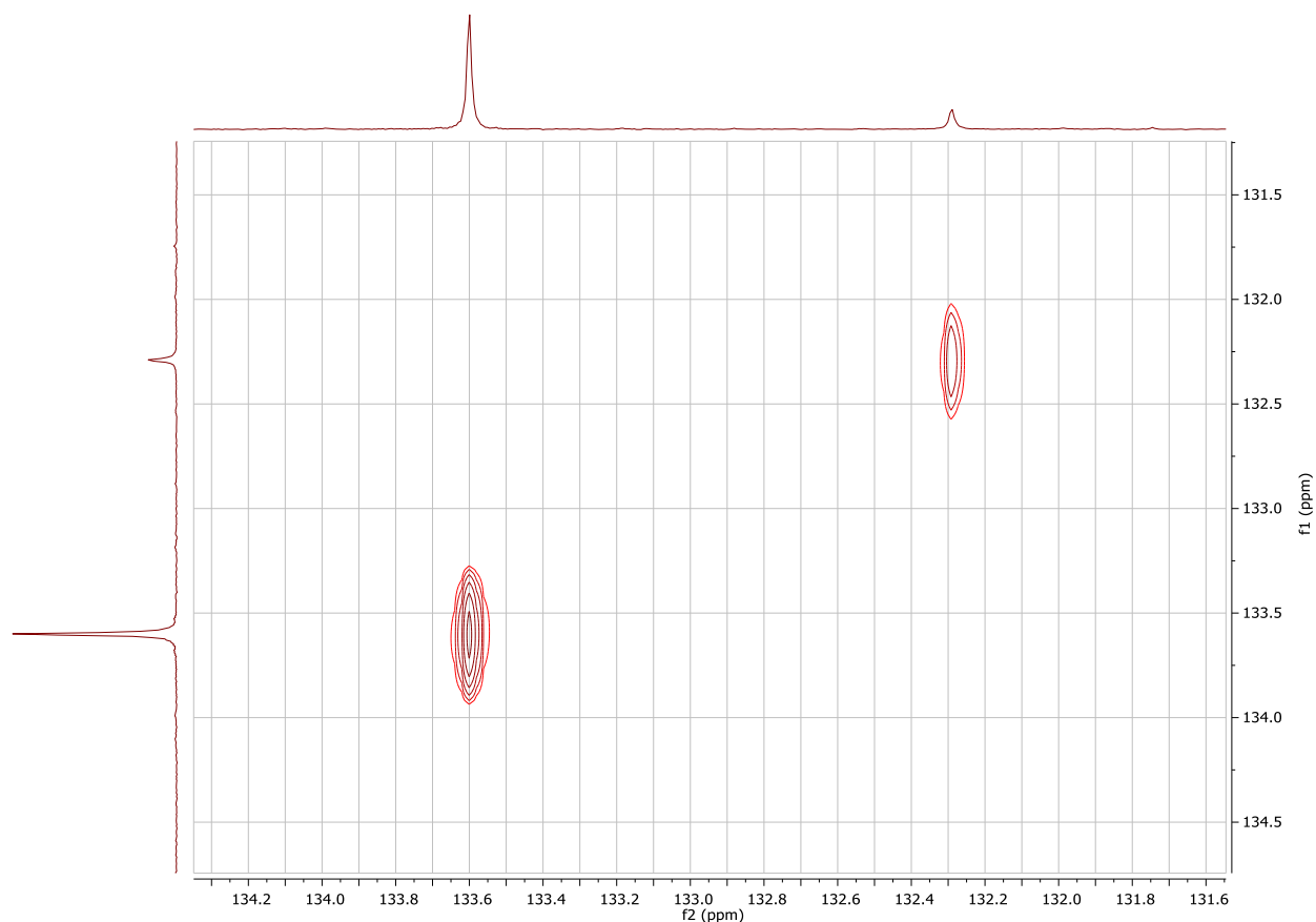
Figure S6. ^{31}\text{P} - ^{31}\text{P} EXSY NMR spectrum of the catalyst resting state (mixing time = 0 ms).
