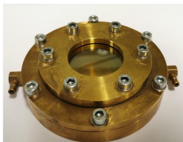
Supplementary Figure 1. Reaction cell: A photograph of a reaction cell for laser-induced nitrogen fixation.
