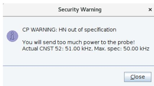
In this way, each pulse sequence has its own personalized security which is adapted for its use and to the probe specification :
