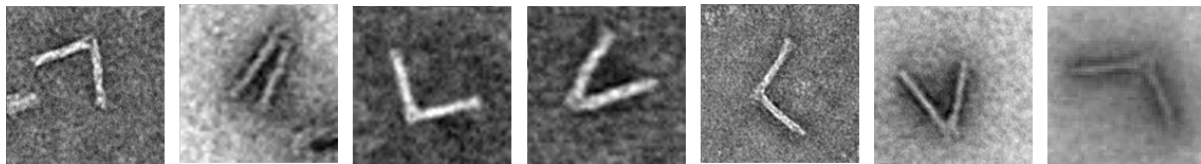
Figure S7 Heavy metal Uranyl formate staining process to TEM grid gives random image contrast behavior.
