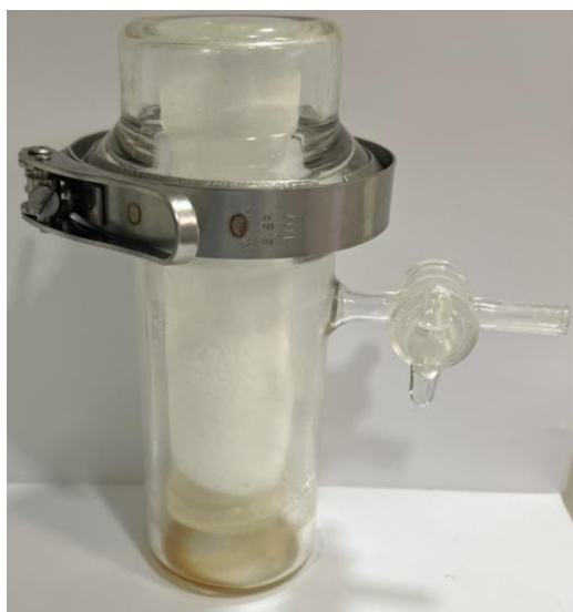
Figure S73. Sublimation kit for depolymerization of 10.0 g of PLLA using Sn(Oct) 2 and GEO ([Sn(Oct) 2 ] 0 : [OH GEO ] 0 : [PLLA] 0 0.0625: 20: 10000, 160 °C)
