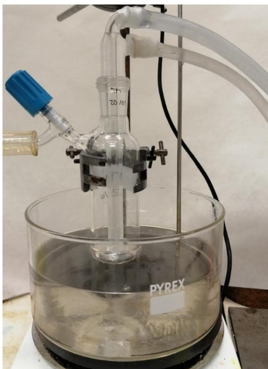
Figure S23. (left) Setup used for depolymerization-sublimation of PLLA to LA. (right) Lactide collected on a cold finger
