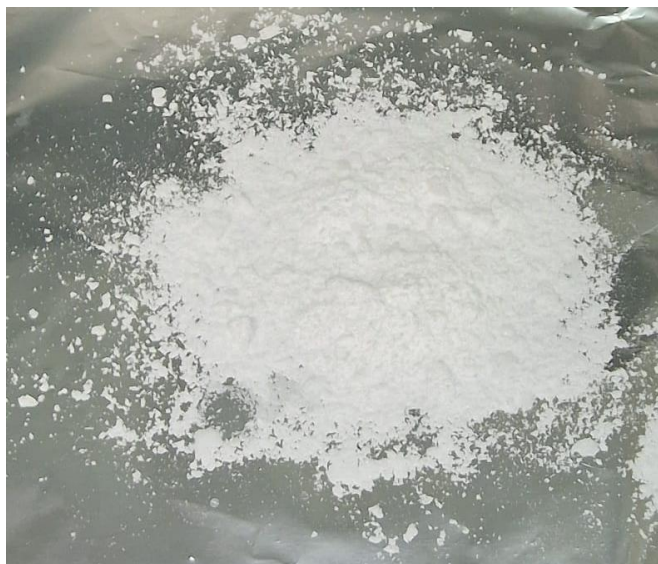
Figure S72. Representative L -LA isolated from depolymerization of PLLA using Sn(Oct) 2 and GEO catalyst
