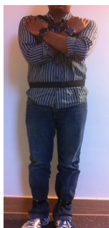
Figure 5 – A man wearing the small Opal sensors which are worn by study participants during the gait analysis.
