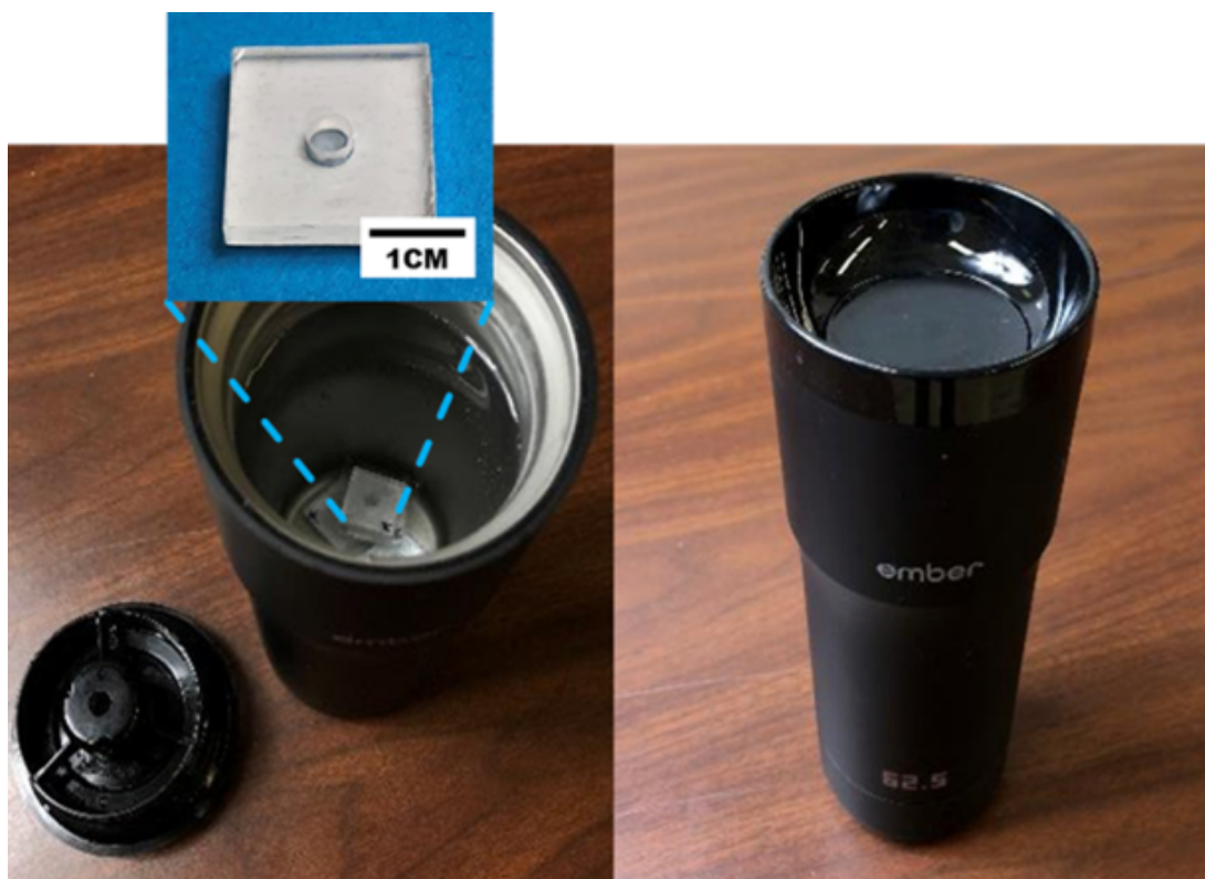
Figure S5. Photographs of a commercially available coffee mug used as a water bath for isothermal amplification in the format of endpoint detection. The mug is powered by a rechargeable battery and controlled using a smartphone App. The subsequent detection of the amplicons of RT-LAMP is achieved by adding 0.5 \mu\text{L} of 10,000X concentrate SYBR green dye at the end and the color change can be observed by the naked eye if MAYV is present. To enhance visualization, a blue LED flashlight is used to illuminate the reaction mixture, and fluorescence signal would be observed. A no-template control is included, as a negative control, in each test. The test results, i.e., the image of detection units, are captured using a smartphone camera and the presence/absence of the amplicons after RT-LAMP is confirmed by gel electrophoresis.
