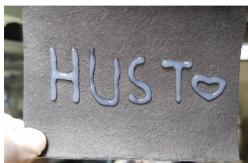
Figure S4 Photographs of PLG hydrogel after injection. The photos demonstrate the injectability and self-healing ability of the PLG gel.
