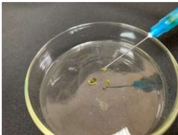
Fig.S1 Image of the HASPy hydrogel injected through the syringe with a needle
