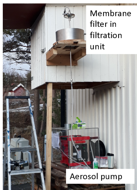
Supplementary Figure 9: Experimental set-up with aerosol pump and filter unit mounted at ~ 2 m above ground close to the coast.
