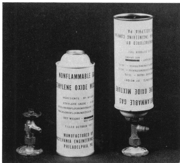
Figure 1. Can holder, aerosol can, and holder attached to can in operating position.
