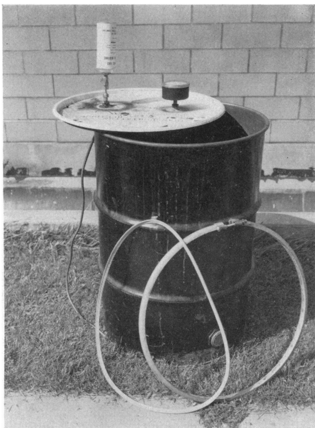
Figure 3. Drum modified for gaseous sterilization
