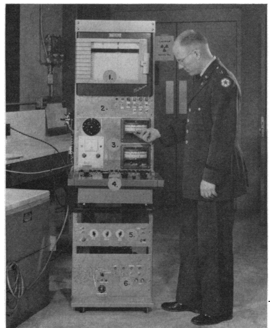
FIG. 7. Control panel. 1. West strip chart recorder; 2. master control panel; 3. temperature control panel; 4. K3 potentiometer; 5. power supply; 6. master power control panel.
