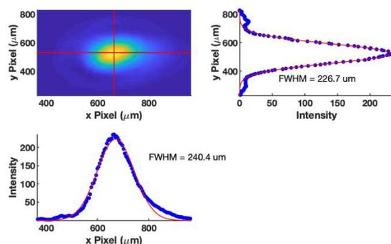
**Figure SI-2:** Gaussian fits to the excitation pulse size as measured on a CCD camera at sample position
