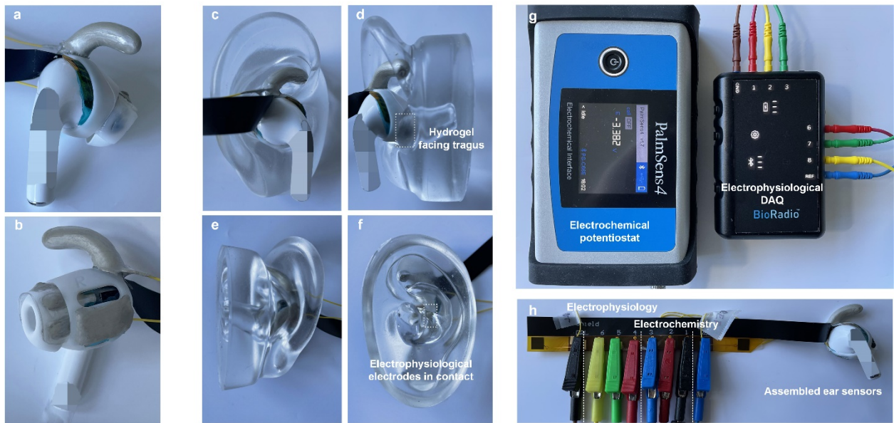
Supplementary Fig. 2 | Assembled in-ear integrated sensors, insertion demonstration, and backend electronic connections. a–b. Images of assembled in-ear integrated sensors on the earphone from different angles. c–f. Images of the in-ear integrated sensors inserted into an ear phantom from different angles. g. Instrumentations used for electrophysiological and electrochemical signal acquisition. h. Connection of ear sensors fPCB to the backend acquisition systems.
