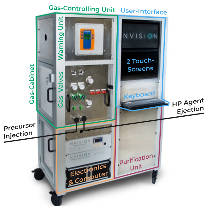
Caption Figure S1: Schematic of the automated polarization process and photograph with description of key elements of the polarizer prototype.
