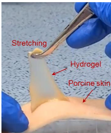
Figure S11. Optical image of the hydrogel tough-bonded to a porcine skin surface.
