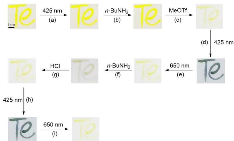
Supplementary Figure 151. The manipulation of writing of Z-5 (10 mM, \text{CHCl}_3 ) as letters “Te” on a filter paper with photoswitching, dynamic nucleophilic substitution, and dynamic imine chemistry. (a) 425 nm, 10 s; (b) aqueous n -BuNH 2 (40% w/w), 20 s; (c) MeOTf, 10 min; (d) 425 nm, 20 s; (e) 650 nm, 4 min; (f) aqueous n -BuNH 2 (40% w/w), 30 s; (g) aqueous HCl (30% w/w), 40 s. (h) 425 nm, 20 s; (i) 650 nm, 4 min.
