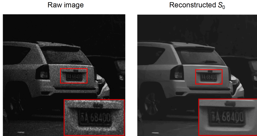
Supplementary Fig. 13 | The reconstructed intensity image S_0 of the pixel-level scene in Fig. 5. The car plate is scaled into the red box. The numbers on car plate are only one or two meta-pixels in width and can still be reconstructed clearly.
