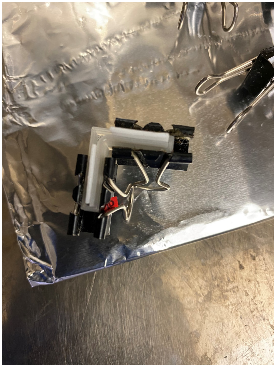
Figure S3. Representative photograph showing programming of a sample into the temporary shape by heating at 55 °C for 5 min and then manually bending to a 90° angle in a bracket mold.
