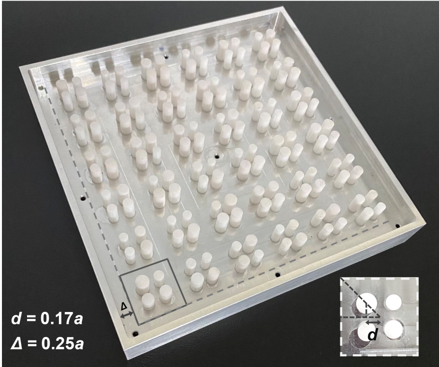
Fig. S3 Photograph of the sample. The boundary of PCs and the air gap is indicated as the dashed line, \Delta = 0.25a is the thickness of the air gap. The lower right panel is a zoom-in picture of the unit cell where d denotes the distances of the dielectric cylinders from the center of the unit cell both horizontally and vertically. The picture shown here is the sample of d = 0.17a with the onsite potential disorder.
