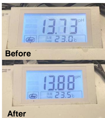
Figure R1. The change of pH value before and after NITRR reaction for 1 hour.
