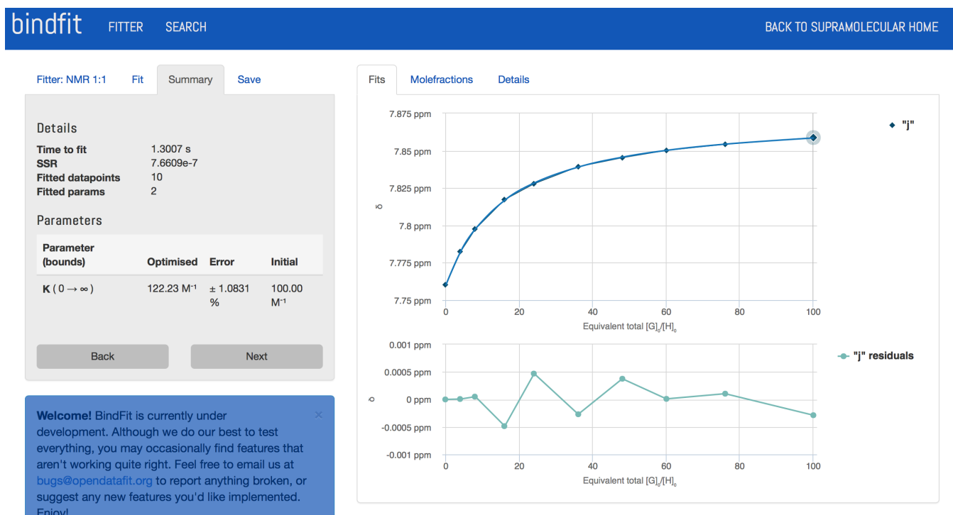
Figure S13: Fitting of H j shift ( \Delta\delta ppm) from S12 using a 1:1 model.
