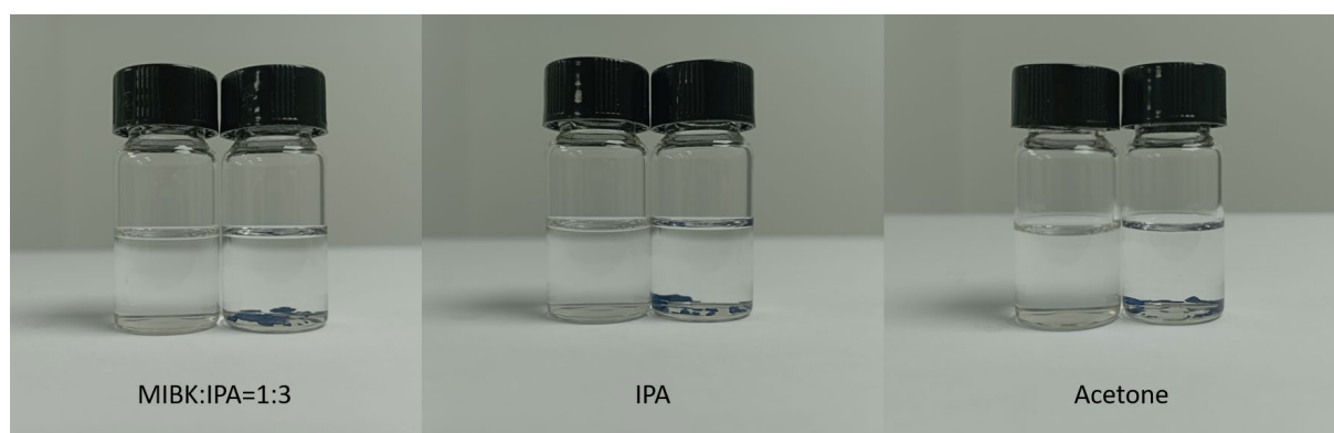
Figure S8. Images of MIBK/IPA, IPA and acetone solvents (left sample in each image) and mixture of TPPS powders with these solvents (right sample in each image), respectively. The images were taken 3 days after adding the TPPS powers into the solvents.
