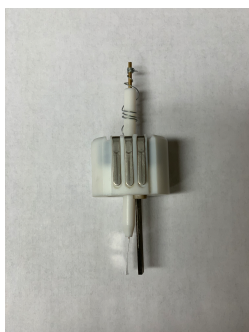
3. Assemble both graphite electrode and Pt electrode.
