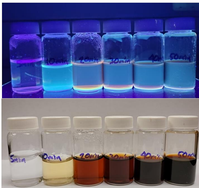
Figure S1. Fluorescence upon UV illumination (top) and suspension colors (bottom) for different batches of PEI-GQD after the synthetic times of 5, 10, 20, 30, 40, and 50 min in a microwave-assisted hydrothermal reaction.
