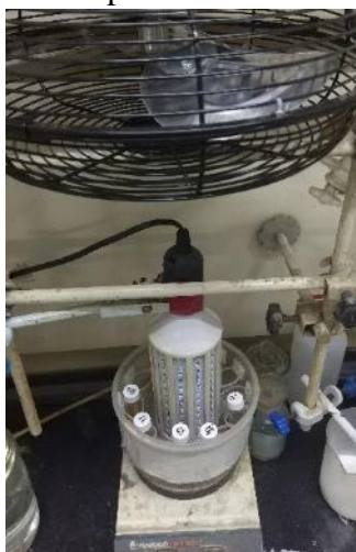
Figure S1 Photograph of the Photocatalytic reactor used for reactions conducted under blue LED irradiation.
