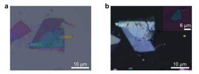
Supplementary Fig.13. Self-aligned process for thinner heterostructure. a, Optical
