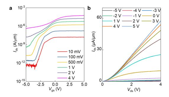
Supplementary Fig. 15. Self-aligned device operated on the SiO<sub>2</sub>. a,  $I_{ds}-V_{gs}$  transfer characteristics of a self-aligned device on SiO<sub>2</sub>. b,  $I_{ds}-V_{ds}$  output characteristics of a selfaligned device on SiO<sub>2</sub>. The thickness of MoS<sub>2</sub> is 14 layers, channel length is around 80 nm.
