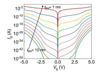
115 Supplementary Fig.14. The simulation results of gate leakage currents with different
