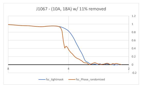
Subsequent local refinement of the receptor alone appeared to substantially improve the quality of the phase-randomized FSC curve, without impacting global resolution.
