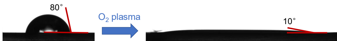
Figure S2. Water contact angles of the surface of LCE in different states
